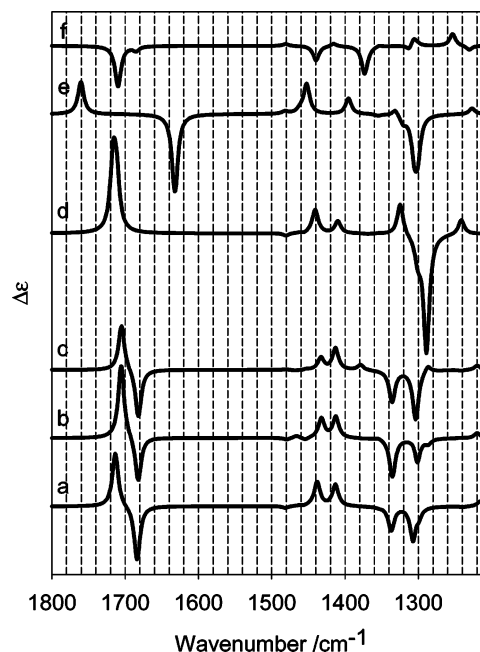
Figure 3. Calculated VCD spectra for different conformers of N -isobutyryl-L-cysteine adsorbed on a \text{Au}_8 cluster. The letters correspond to the structures shown in Figure 2.
